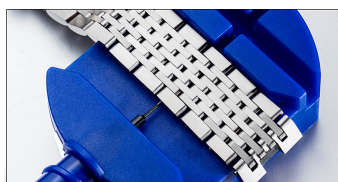
2. Put the bracelet into the slot of the adjuster. Align the needle with the round end.
